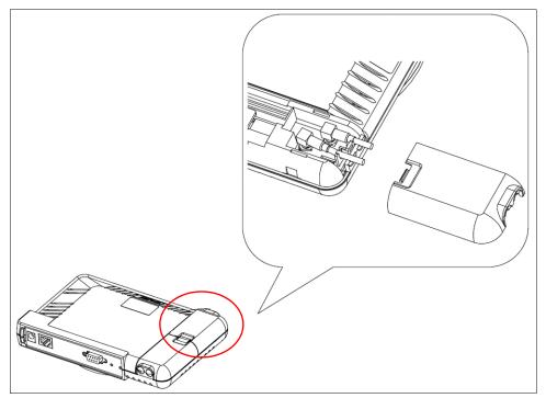
Figure 2-6 Opening the Antenna Compartment
